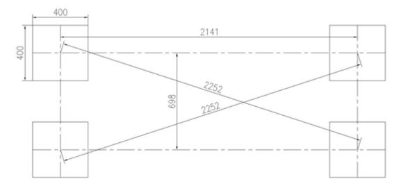
Pour concrete into the hole to form the basic layer of 100mm. And combine the J-bolt with installation mould and put the bolts into the hole. (Refer to the diagram for space and size). Pour concrete of 1:2:3.5 into the hole (concrete mark shall not less than 325#), smooth the surface.
