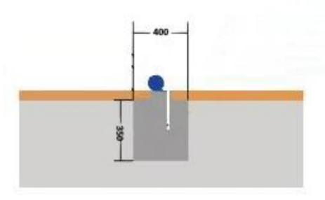
After the concrete is totally hardened, fasten the equipment onto the installed J-bolt with 4\*M12 flat washer, spring washer and nut (see pics below). After installation, check the perpendicularity of the equipment to ground surface with tolerance less than 1/100.
